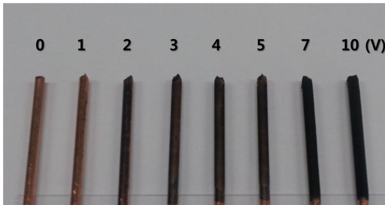
Figure 4-9. Optical image of MGCN foam emitters with various applied voltages. The diameter of a copper wire is 2 mm.
