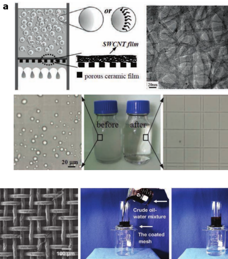
Figure 3-4. (a) Separation of water-in-oil emulsion where oil selectively permeates through CNT film [105]. Optical microscopy images of water-in-oil emulsion before and after filtration. (b) Oil/water separation by using hydrophilic and underwater oleophobic polyacrylamide hydrogel-coated mesh [110].
