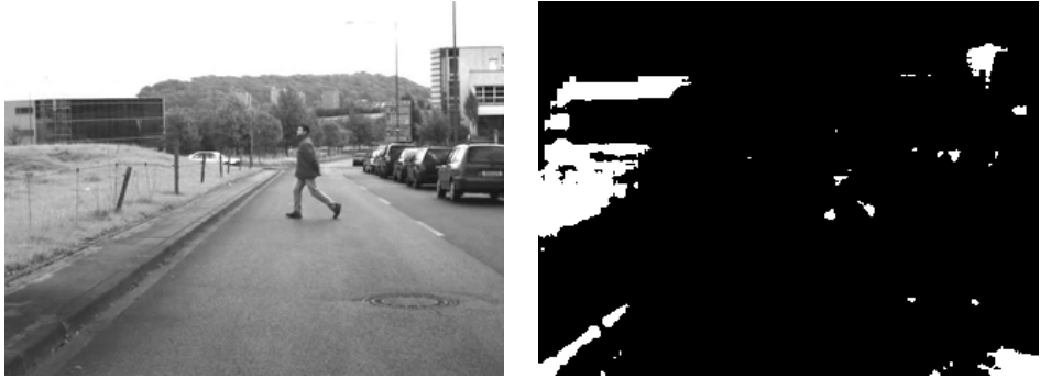
Figure 2.6: The fourth problem from the naive extension of background subtraction for fixed camera: the limitation of homography model in a dashcam.
