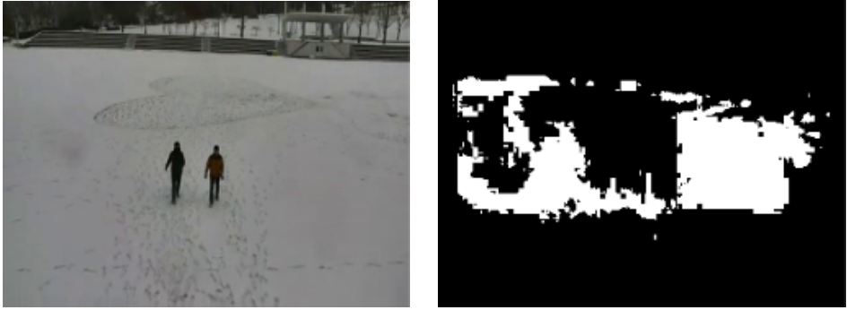
Figure 2.4: The second problem from the naive extension of background subtraction for fixed camera: sudden scene changes such as illumination.
