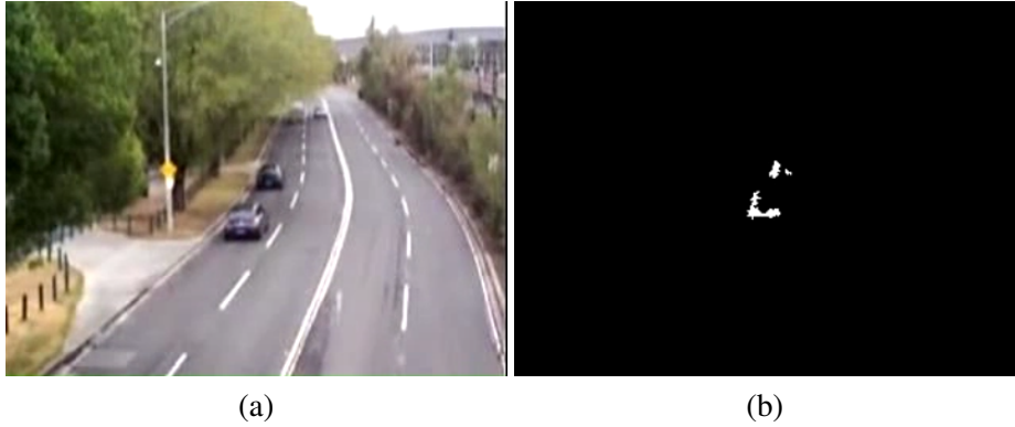
Figure 6.21: The limitation caused by the grid-based modeling. By the perspective of the image, the moving distance on the image is short when the object moves from a distance. Thus, the changed area becomes small, so only a part of the object is detected.
