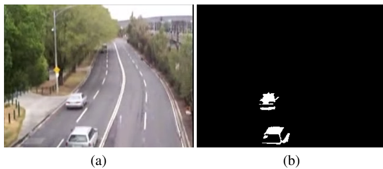
Figure 6.20: The detection result when the proposed method applied without stabilization: (a) input frame (b) detection result.
