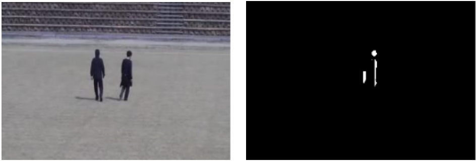
Figure 2.5: The third problem from the naive extension of background subtraction for fixed camera: slow moving object relative to camera movement.
