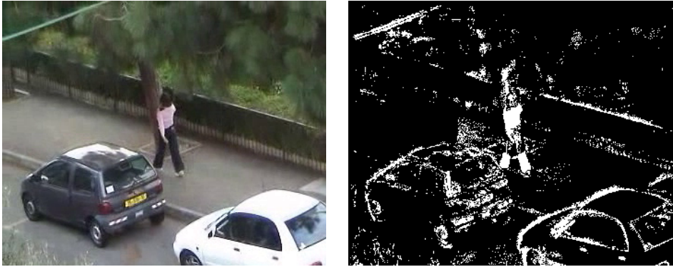
Figure 2.3: The first problem from the naive extension of background subtraction for fixed camera: false positives around edges.
