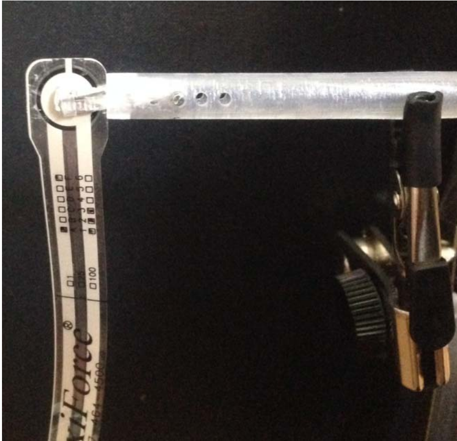
Fig. 3.1 Gripping force measurement experimental setup using Flexiforce.
