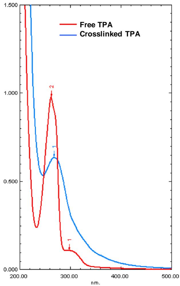
**Figure 7.** UV absorption spectrum of free TPA and crosslinked TPA.
