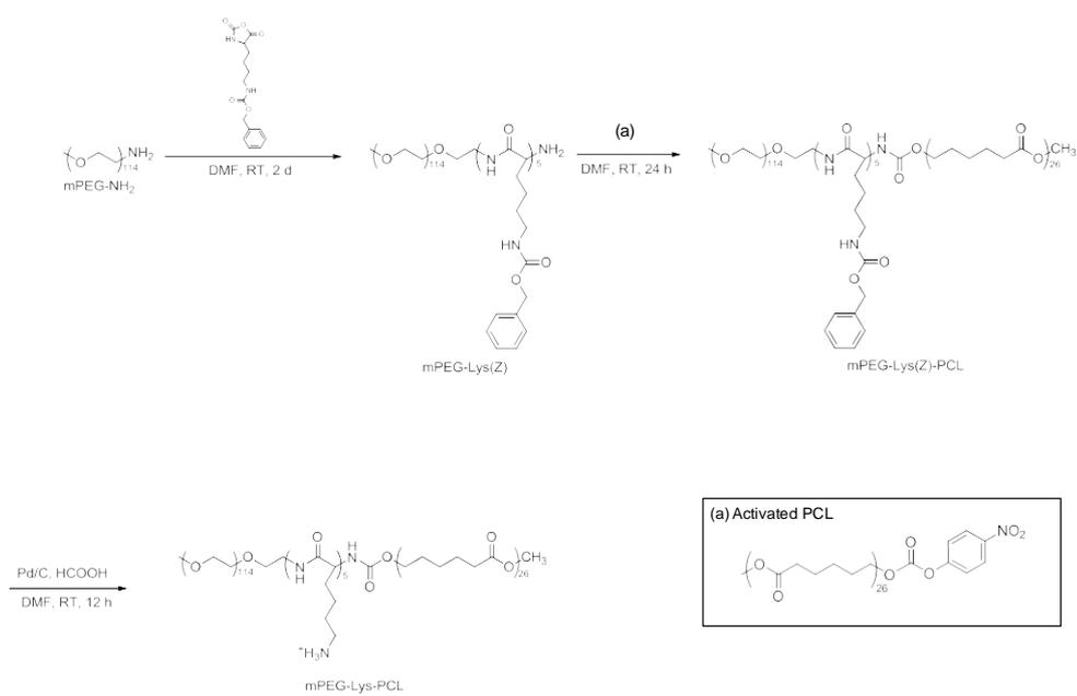
**Scheme 1.** Synthetic procedure of mPEG-Lys-PCL.
