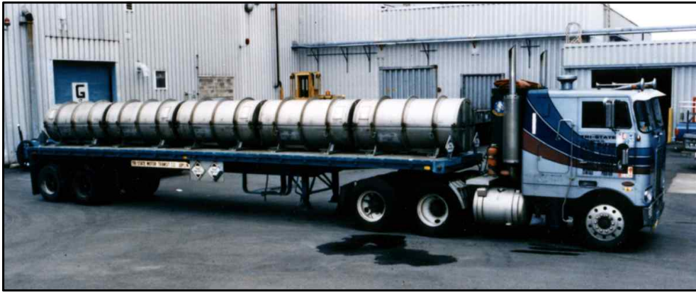
[그림 2-2] Truck shipment of five 2 1/2-ton UF6 cylinders in protective shipping packages
