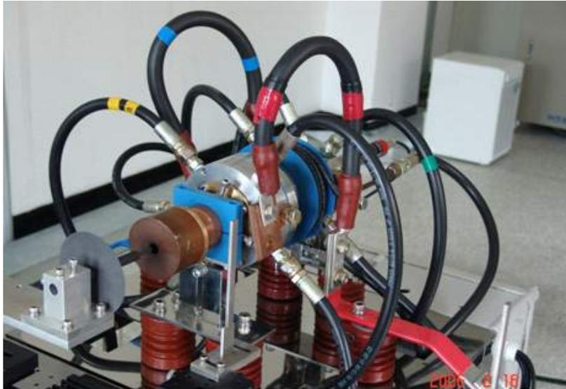
Figure 2.1 150 kW plasma generator
