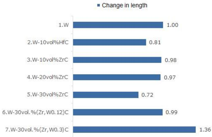
Figure 4.5 Comparison of change in length of each test
