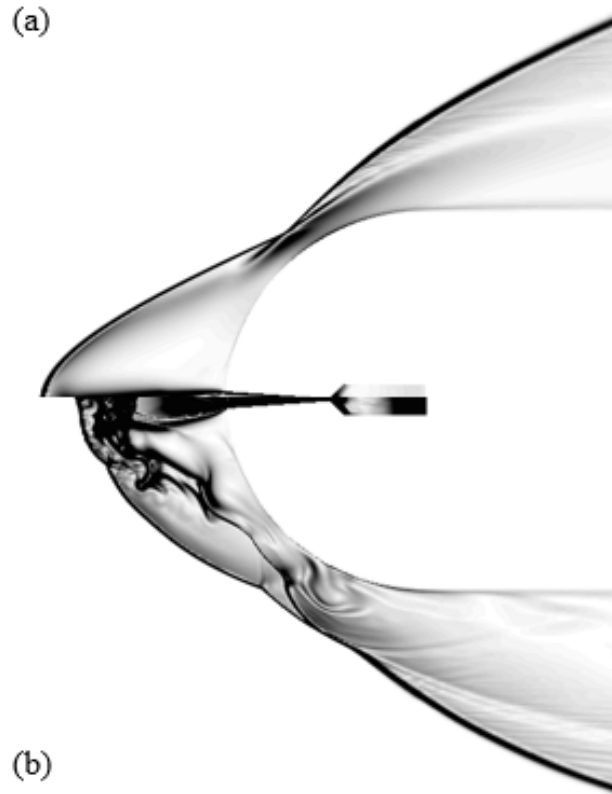
Fig. 22 Local density gradient at higher Mach number of jet
