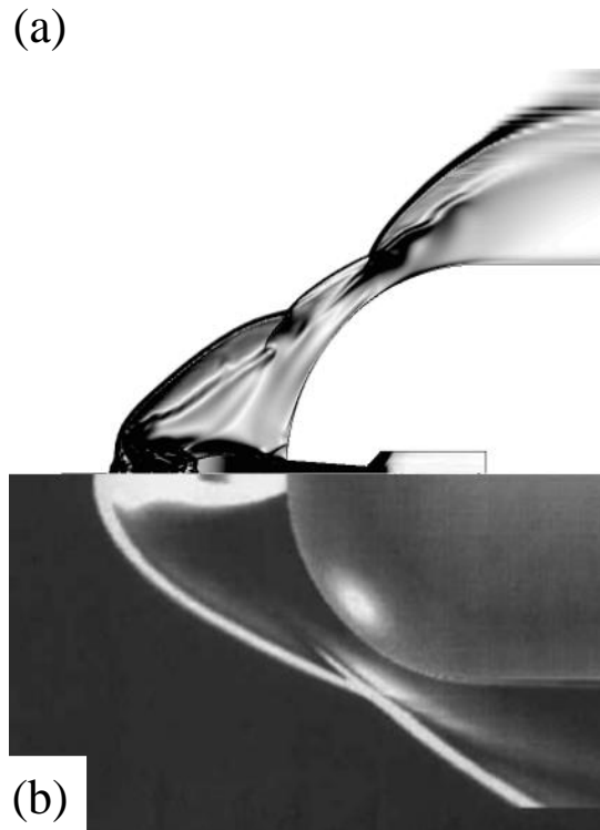
Fig. 9 Local density gradient for LPM (a) Present numerical research
