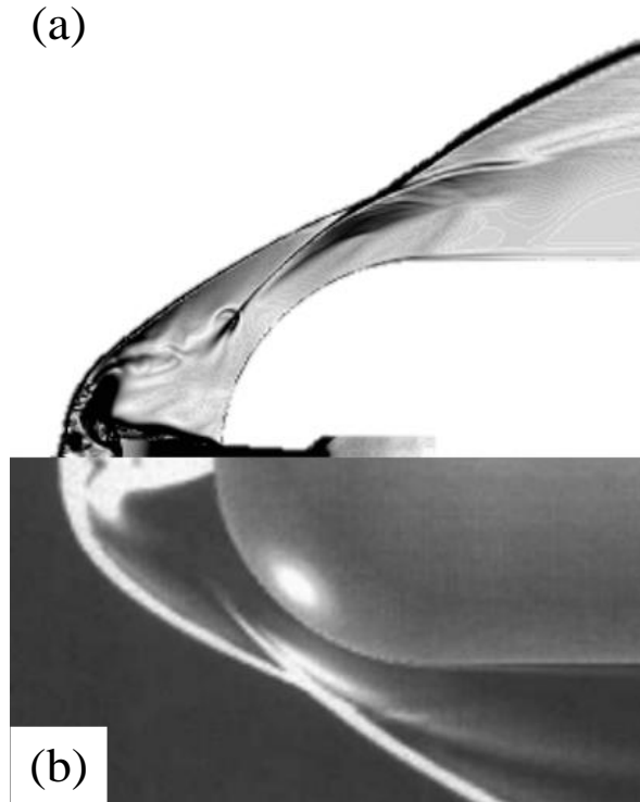
Fig. 10 Local density gradient for SPM (a) Present numerical research (b) Previous study
