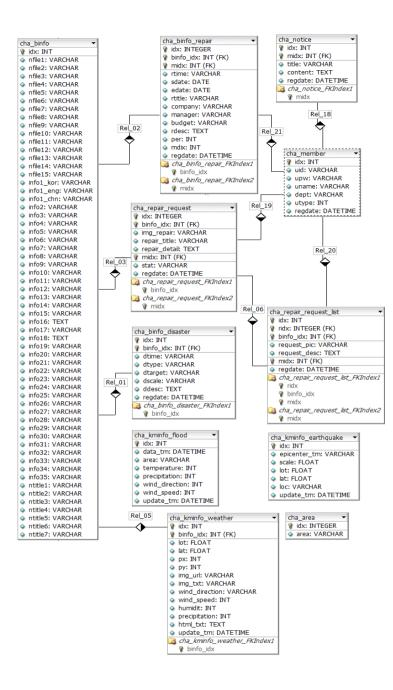
Figure 3-2. Entity Relationship Diagram for Database
