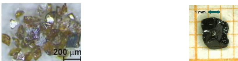
IV-5: Optical microscopy of a batch of 4-1/TCNQ cocrystals used for NEXAFS and HAXPES measurements (adapted from [335] ). Millimeter sized cocrystals used for single-crystal conductivity measurements (pictures courtesy of HUTH group).
