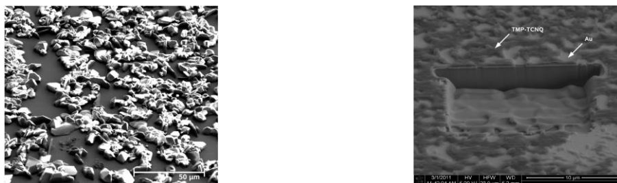
IV-21: Left: SEM image of a low coverage 4-1 /TCNQ film on SiO 2 . Right: SEM image of 4-1 /TCNQ film (dark) on gold (bright). Island growth is observed on both substrates (pictures courtesy of HUTH).
