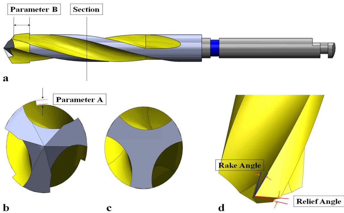
**Figure 3.** Modified drills. (a) Left-right: parameter A was set to 0.15, 0.35 and 0.5 mm, and top-bottom parameter B was set to 7.5, 2.0 and 0.1 mm. (b) High magnification of experimental drill, note the reduced parameter B dimensions that directly contact bone.
