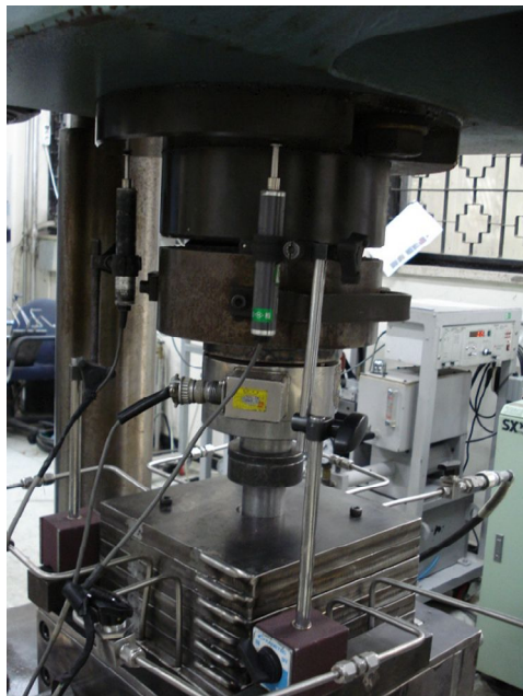
Figure 3.9 Measurement instrument setup: (a) LVDT and load cell setup (b) load test machine
