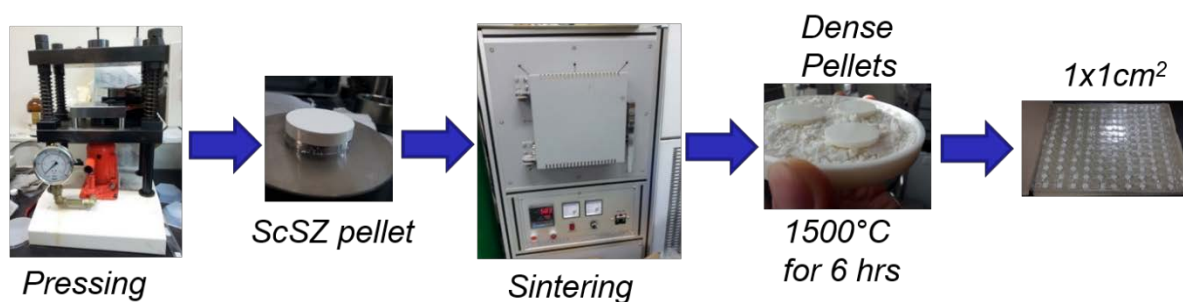
Fig. 5 The process of uni-axial pressing of ScSZ powder followed by sintering and machining
