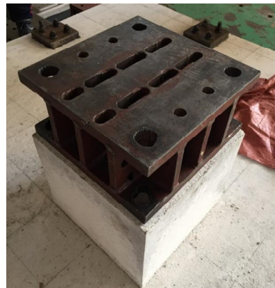
(c) Steel jig anchored at column
