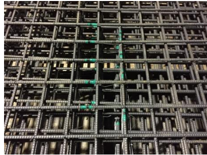
(b) Strain gage installation
