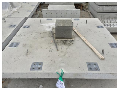
(h) Completed RC specimen
