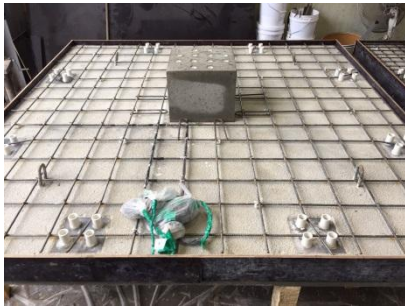
(c) Rebar, strain gage installation
