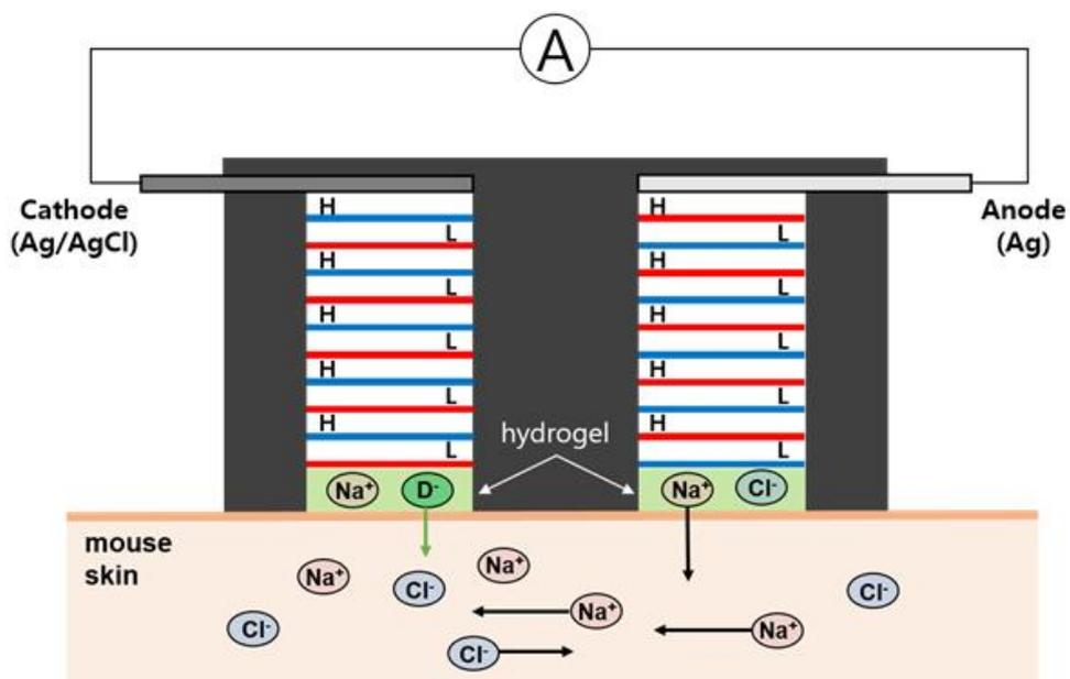
Fig. 11. The schematic image of RED patch with the electrodes to measure the current during *in vitro* and *in vivo* penetration tests.
