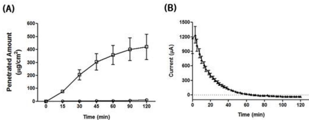
Fig. 14. *In vitro* penetration test of 2% RIS (w/v) using GEL (○) and RED patch (□). The graphs represent the cumulative amount of RIS with the administration time (A) and the current response of the RED patch during *in vitro* penetration test (B).
