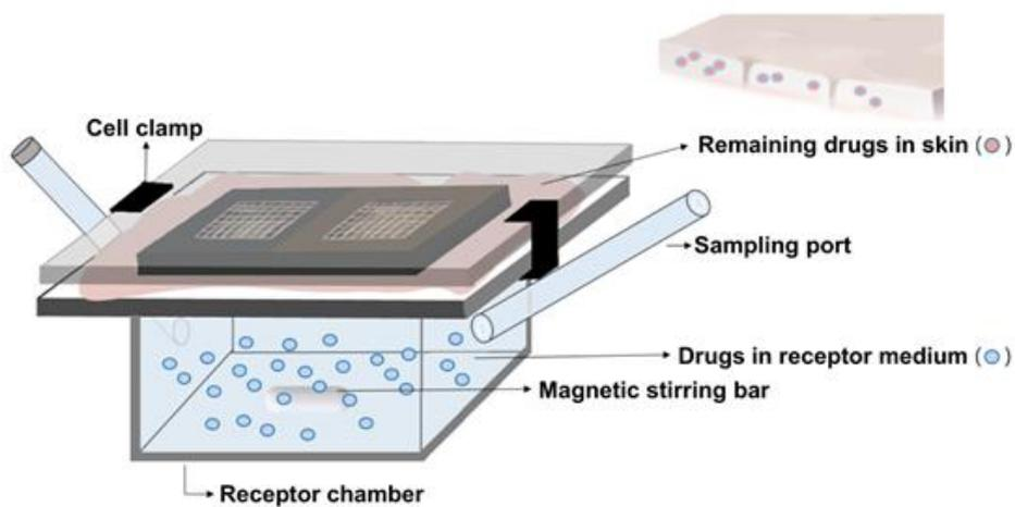
**Fig. 8. Schematic images of the modified Franz diffusion cell for *in vitro* test using the RED patch.** The Franz cell were sustained under a constant condition (37 °C , 200 rpm stirring). The residual amount of drug in the skin and the penetrated amount of drug through the skin were measured over administration of drug.
