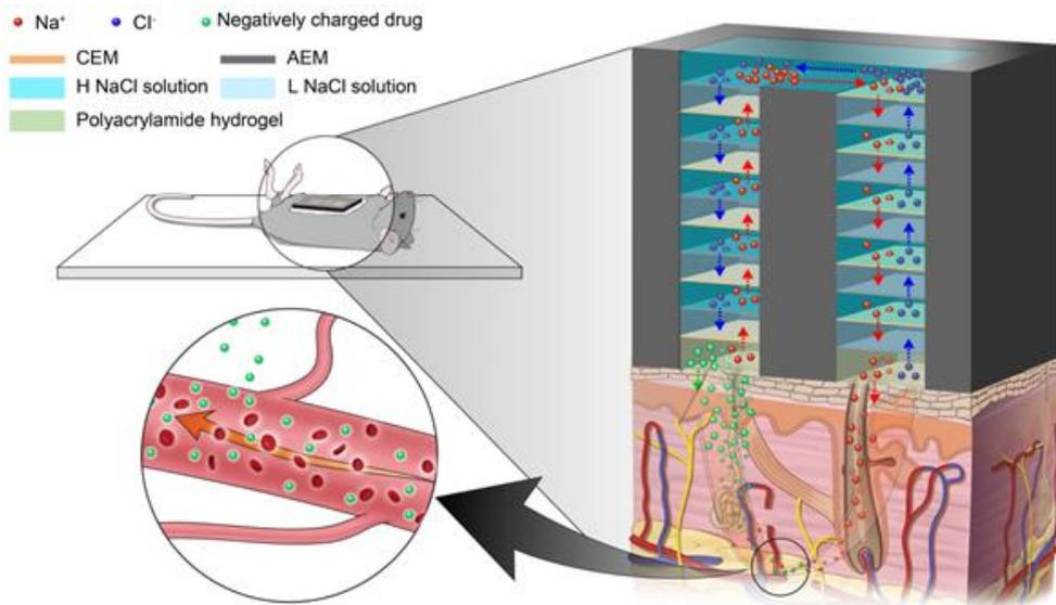
**Fig. 7. A new type of transdermal drug delivery driven by the salt gradient via RED system. Schematic representation of the RED patch attached on the mouse skin. Na<sup>+</sup> and Cl<sup>-</sup> in the RED system move from the high concentrated (H) NaCl solution to low concentrated (L) solution through ionexchange membranes.**
