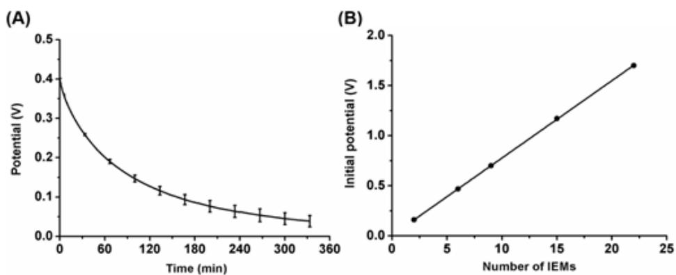
**Fig. 12. Electrical properties of the miniaturized RED patches.** Potential changes of RED patches with  $9.79 \text{ k}\Omega$  external resistor (A). Initial potentials obtained after injection of NaCl solutions (0.017 and 0.51 M NaCl) alternatively over the number of IEMs used in the RED (B).
