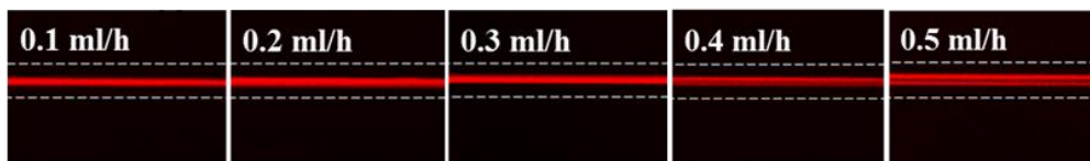
Figure 5.6. Flow rate effect for particle focusing location (a) in 100 ppm HPC solution, and (b) in 2000 ppm PEO solution.
