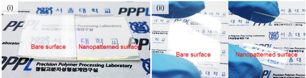
Figure 3.3.9. Optical photograph for comparison of surface reflectance between the bare and the nanopatterned surface under (i) solar light and (ii) fluorescent light.
