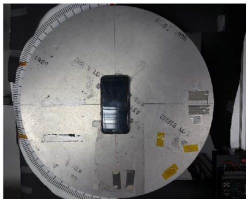
Figure 2-13. Gyro angular velocity controlled turn table
