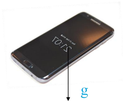
Figure 2-6. Gravity to Z – axis
