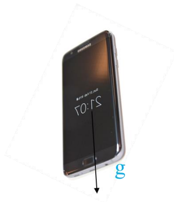
Figure 2-7. Gravity to Y – axis
