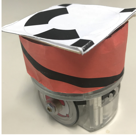
Figure 5.5: An image of e-puck mobile robot used for the real world experiment. The robot is two wheel-based mobile robot with 2 wheels, 10 light-emitting diodes, 8 infrared sensors, 3 microphones, and 1 speaker.
