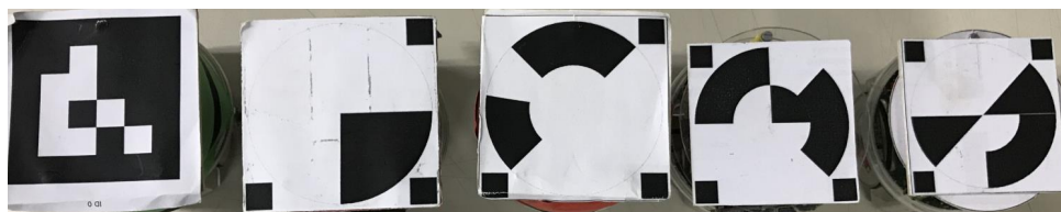
Figure 5.4: Five tags used for catching position and orientation information of the robots.
