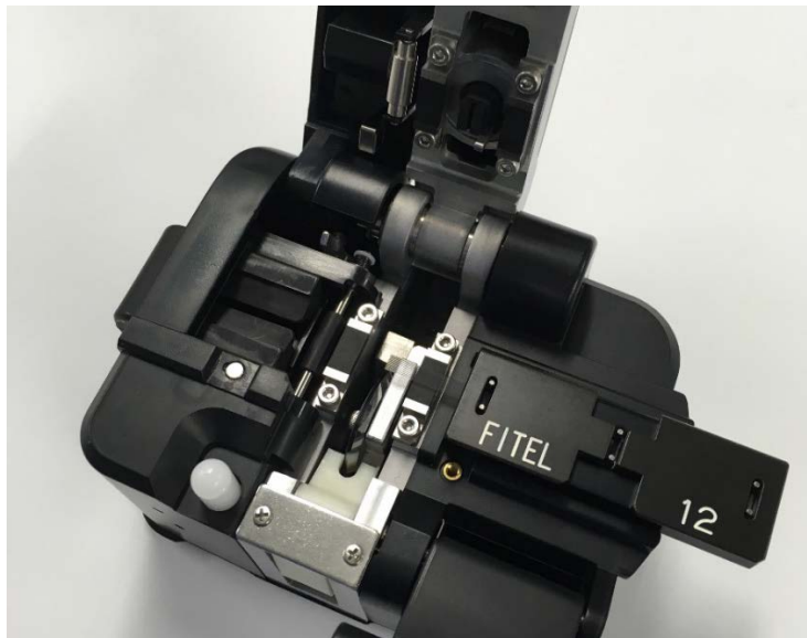
Figure 3.6 Optical image of the high precision fiber cleaver and ribbon holder.
