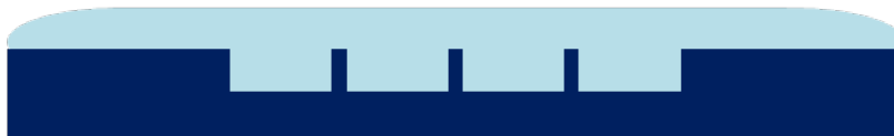
(c) Filling the cavity with glass via anodic bonding and subsequent annealing.
