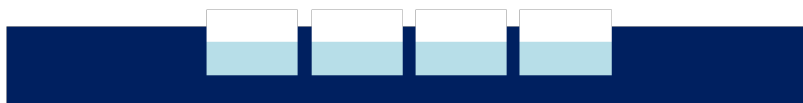
(d) Planarization of BSG over surface of silicon wafer and leveling using HF wet etch
