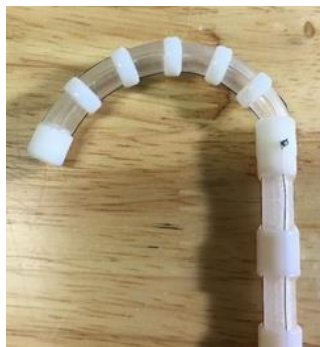
Figure 4.12: Steerable catheter with SMP joint. (a) Backbone ring for SMP tube (Left:Isometric view, Center:Front view, Right:Side view) (b) Steerable catheter with SMP joint (c) Bending test of the 1st joint (d) Payload test of the 1st joint
