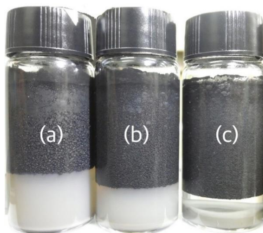
Figure 4.2. Visual demonstration of the o/w emulsion phase formed for solid concentrations of (a) 0.31 wt%, (b) 0.62 wt%, and (c) 1.25 wt% in +140 fly ash samples.
