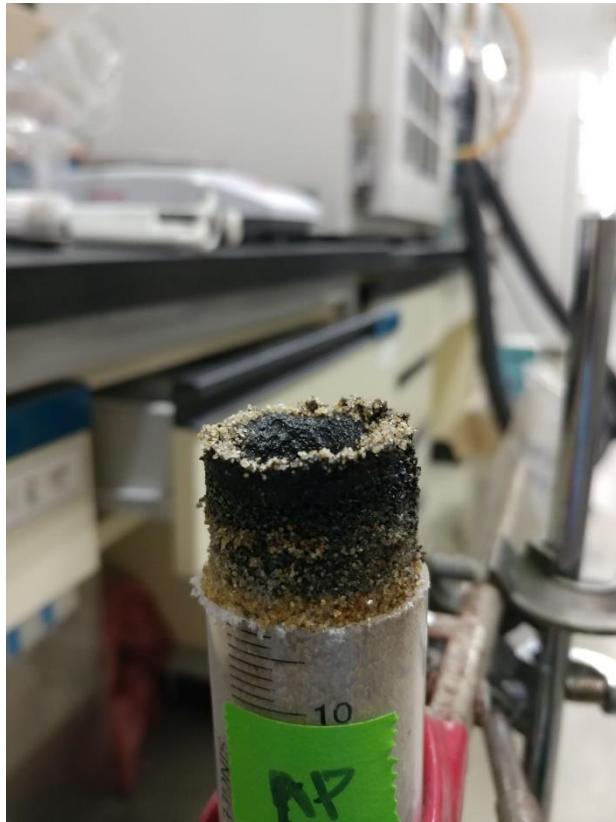
Figure 4.9. Appearance of the sample pushed up for surface-scraping (for the case of AEL OHA).
