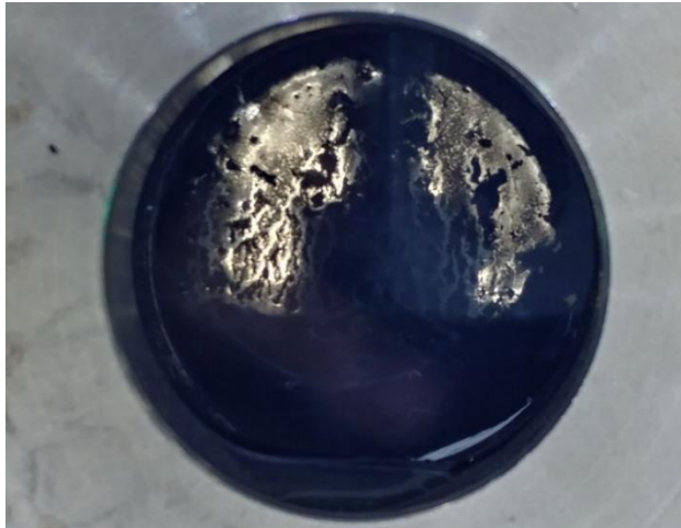
Figure 3.28. When 5 wt% of fly ash (50% LOI) with 0.5 ml of turpentine oil was mixed with supercritical CO 2 , no foam was observed.
