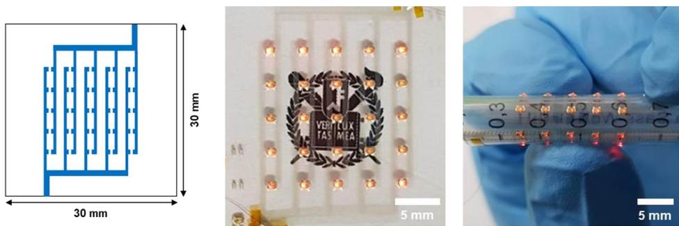
Figure 4.13 5×5 LED arrays on the AgNW-transferred PEDOT:PSS electrode circuits. A circuit diagram (left), a flat state (middle), and a bending state (right).
