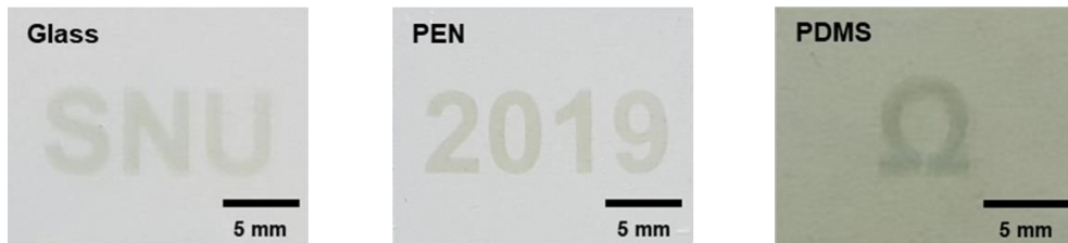
Figure 4.5 Various-shaped AgNW-transferred PEDOT:PSS films on glass, PEN, PDMS substrates.
