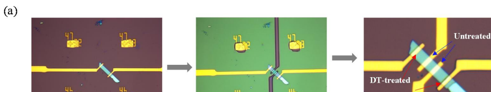
Figure 4.5 (a) Optical images of asymmetric MoS 2 FETs during the fabrication process.
