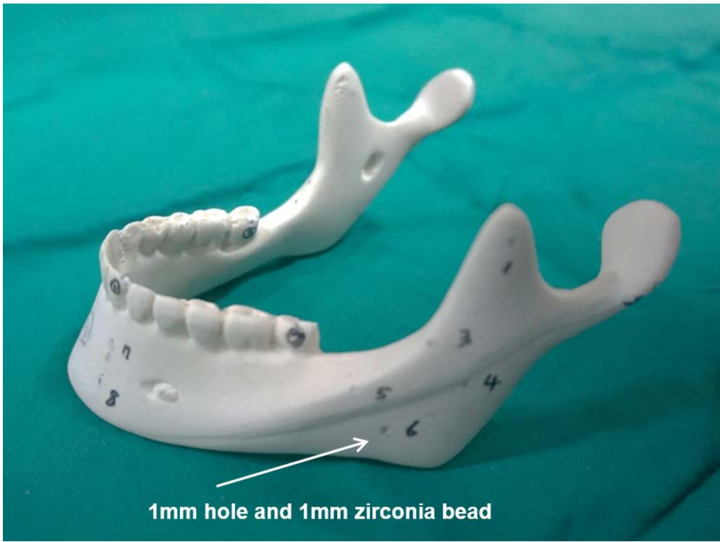
Figure 4. A prepared mandible model for testing the fiducial localization error and target registration error. A 1 mm diameter hole was made and a zirconia sphere bead with 1 mm diameter was put in the hole.
