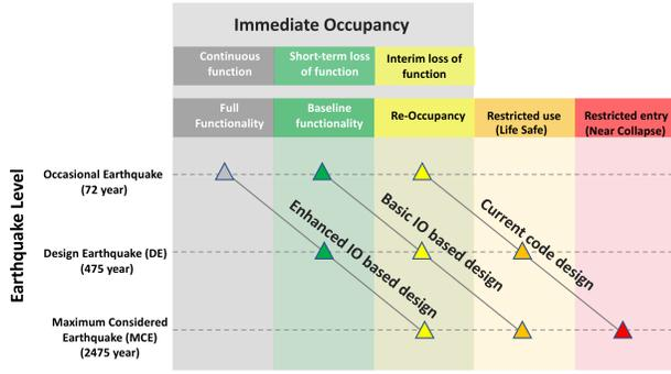
Figure 1 Example of Immediate Occupancy (IO)-based design and current code design
