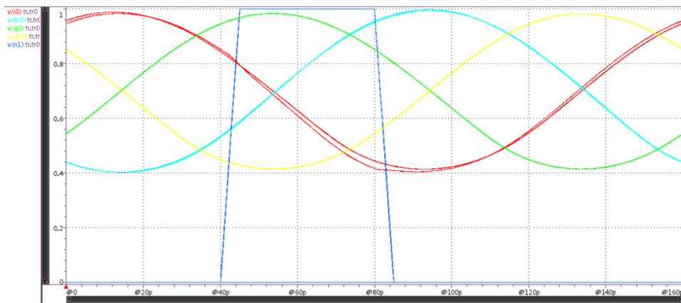
Figure 3.25. simulation result of the asymmetric distortion of output clock.
