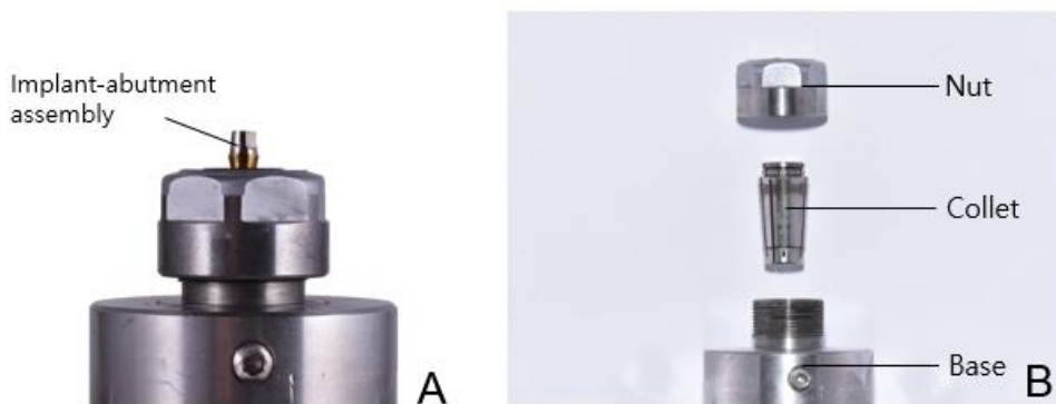
Figure 5. (A) Implant–abutment assembly clamped with an implant holder (Nikken Kosakusho Works, Osaka, Japan), (B) Detailed internal structure of the clamping tool (Nut, Collet, and Base).
