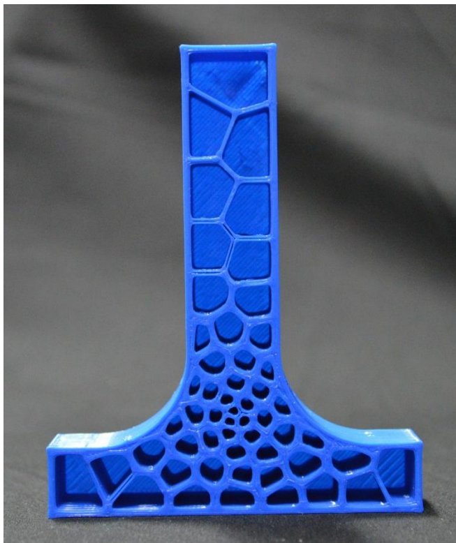
Fig. 47. T-shaped part with designed inner structure
