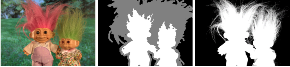
Figure 3.2: Example of image matting. From left to right: Color image, input trimap, and result of matting respectively. The white, black, and gray regions in middle image represent foreground, background and unknown regions, respectively.
