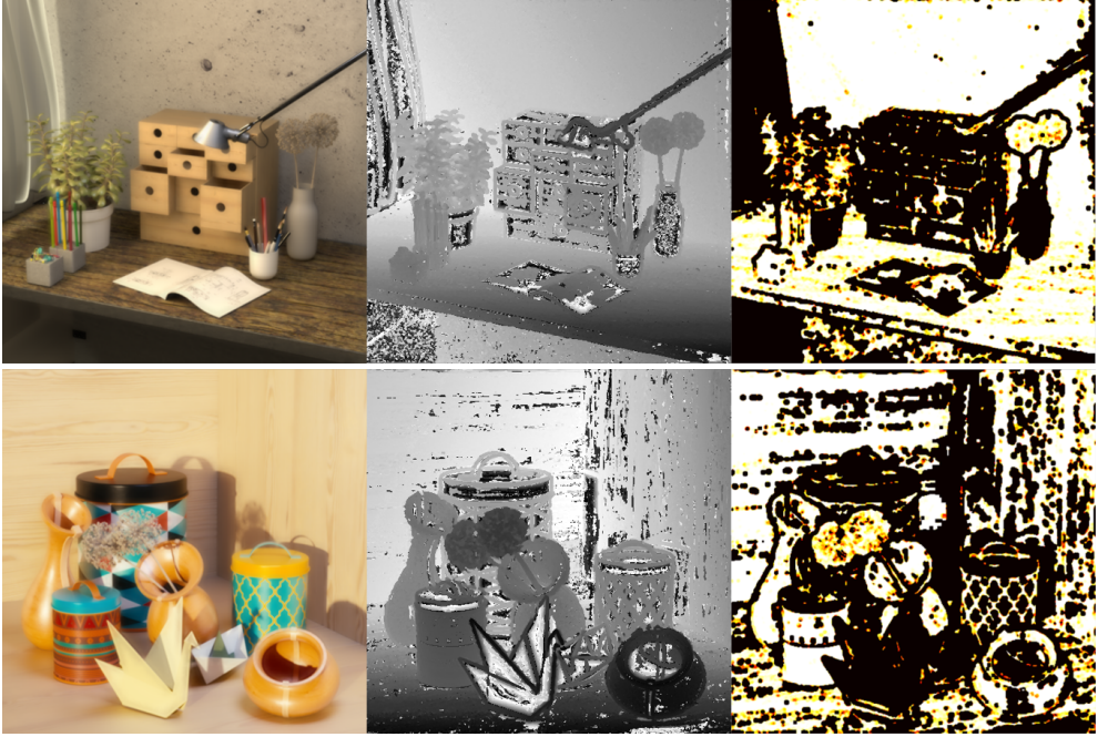
Figure 3.7: Confidence map of selected synthetic data from 4D light field benchmark [56]. From left column to right column are all-in-focus images, the estimated initial depth images; and the corresponding confidence maps, respectively. The confidence map indicates that brighter pixels have higher confidence levels.
