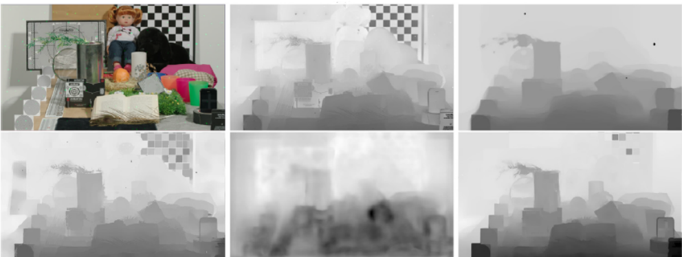
Figure 5.7: Comparison of recovered depth image. From top left to bottom right: all-in-focus image, the results by Tseng [12], Moeller [3], Javidina [13], Hazirbas [14], and ours, respectively.
