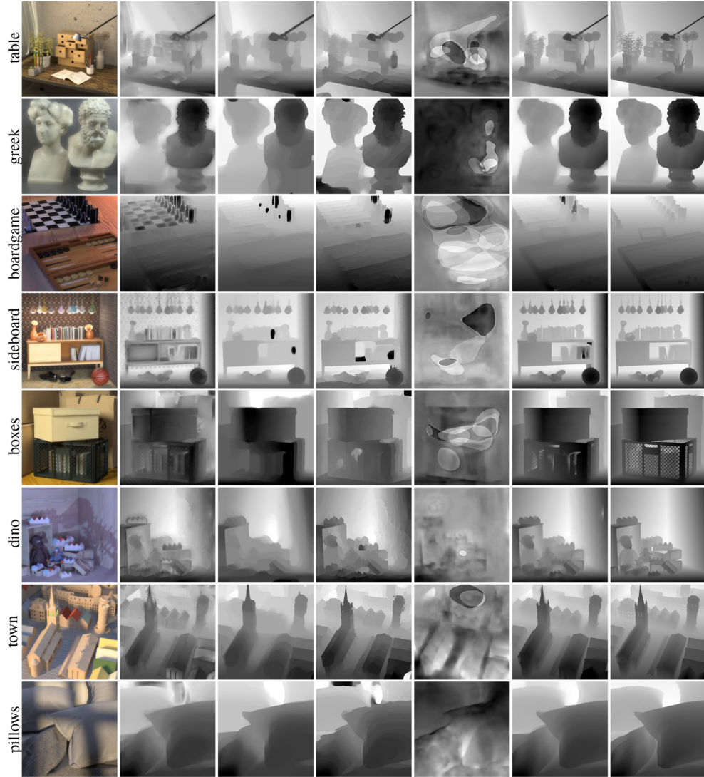
Figure 5.1: Comparison results of recovered depth images. From left to right: all-in-focus images, the results by Tseng [12], Moeller [3], Javidnia [13], our algorithm, and ground truth, respectively.
