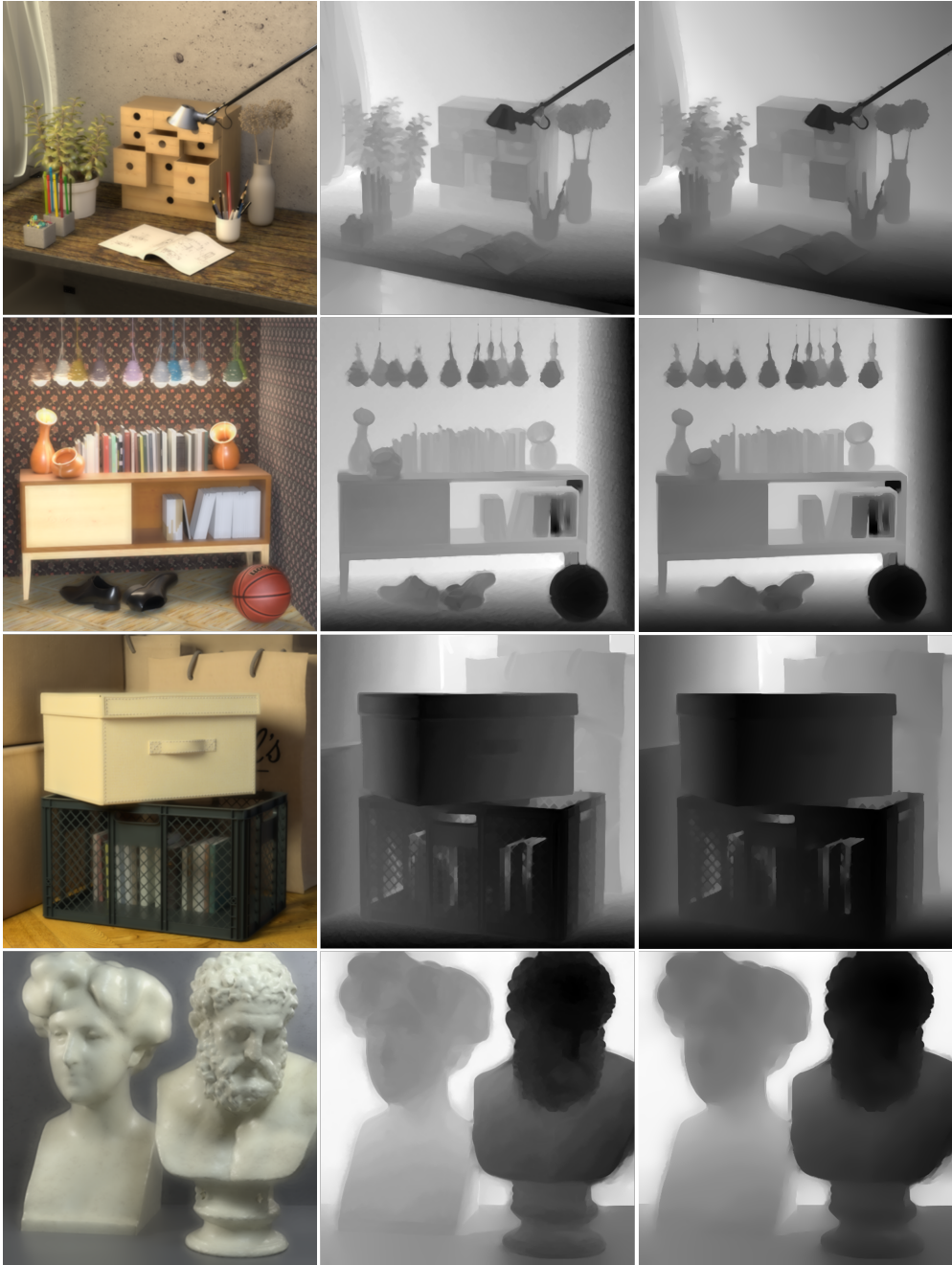
Figure 4.4: Refinement results using proposed edge-preserving method. The left column images are the all-in-focus images. The middle column images are reconstructed depth images using the proposed reconstruction method. Images on the right column are refinement results.
