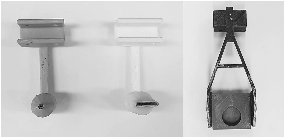
Figure 3.10: Jigs produced by 3D printer (point, line, open type from left)
