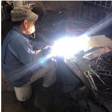
(a) Rebar processing
