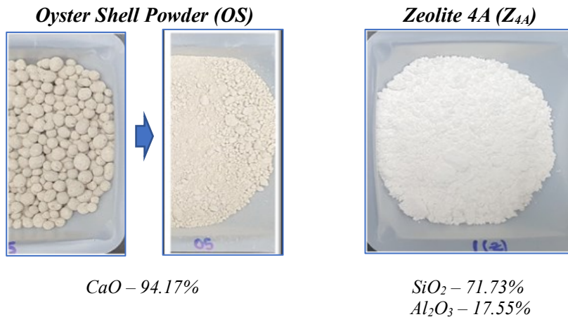
Figure 3.2 Characteristics, texture and porosity (by SEM analysis), quantity analysis by XRD and main chemical compounds by XRF of the binders used in the second evaluation
