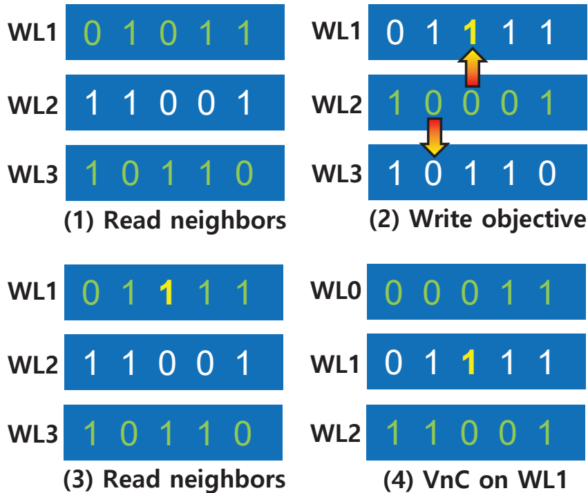
Figure 2.4: Step-by-step illustration of VnC. The yellow colored number represents the flipped bit exposed to WDE.
