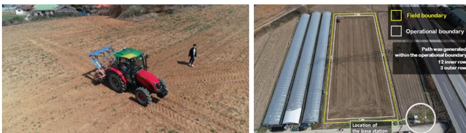
Figure 3. View of autonomous tractor developed by TYM, unmanned solution, and SNU and field test.
