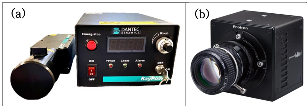
Figure 16. Measuring devices for PIV system ((a): Continuous laser; (b):
