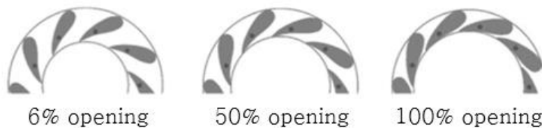
Figure 2.1 Flow control through nozzle angle adjustment using VGN
