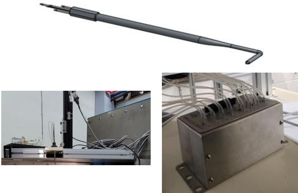
Fig. 4. 5-hole probe (top), 2-axis translation stage (left), and pressure scanner (right)
