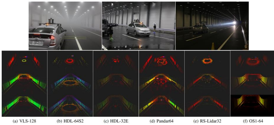
Figure 1.4. Test environment and result of LiDAR shape in dense fog
