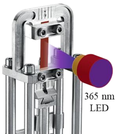
Figure 20. Scheme of the thermal properties observe system constructed with DMA and light source.
