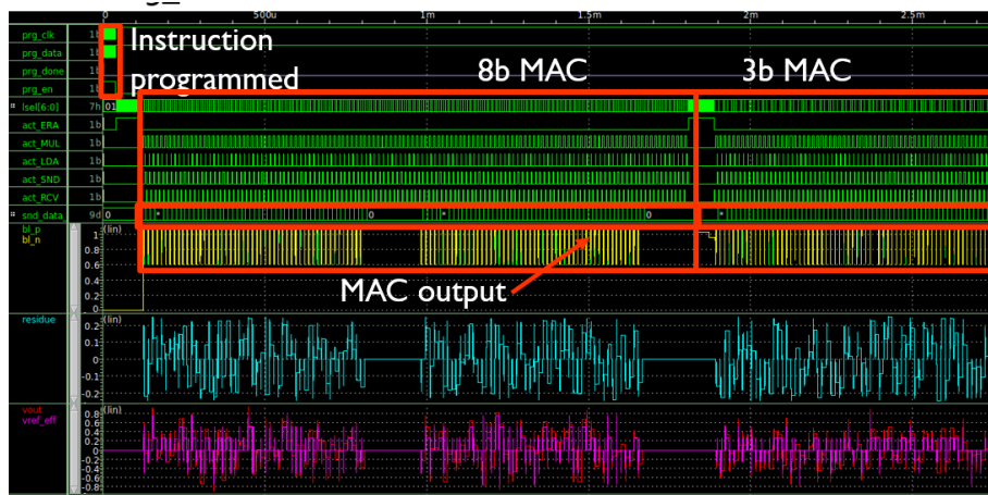
Figure 5.3. The instruction code and simulation result of the 05_mac instruction scenario.
