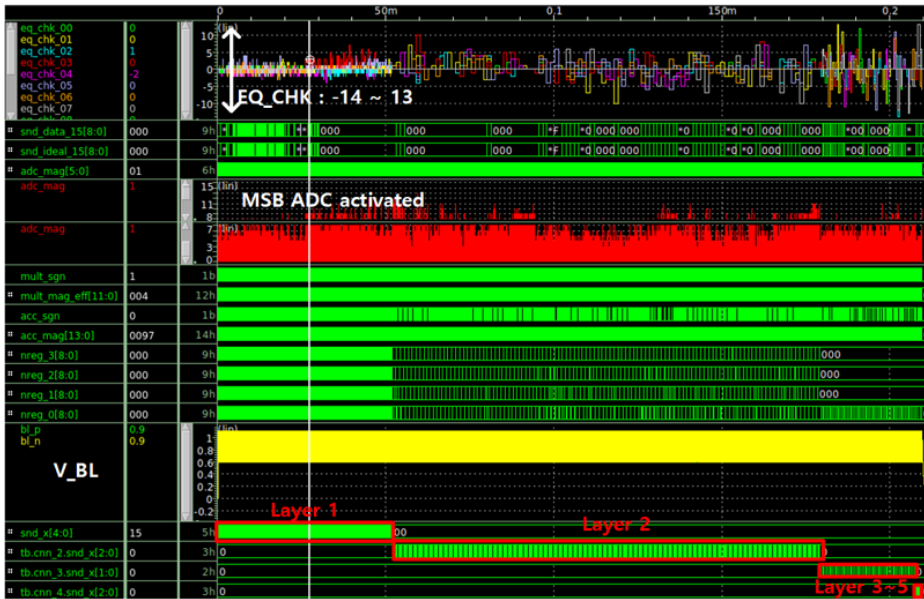
Figure 5.8. The XMODEL simulation result for the CIFAR-10 CNN example with the 9-bit weight precision configuration.
