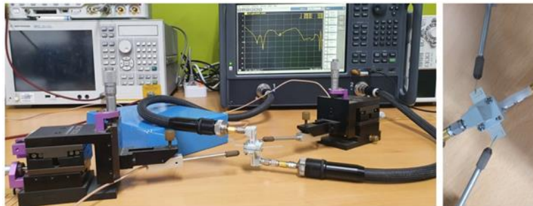
Figure 3.15. Experiment setup (a) Schematic block diagram of the measurement setup, (b) Photograph of the measurement setup; (c) Photograph of the probe tips contacted with the electrodes for biasing the MEMS cantilevers.
