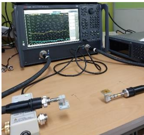
Figure 5.15. Photographs network analyzer and waveguide setup
