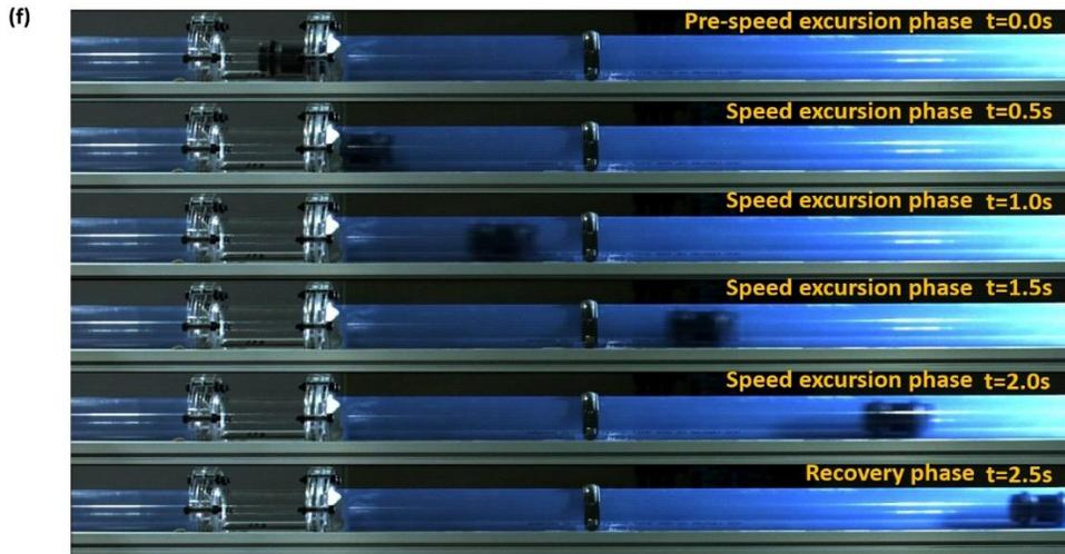
Figure 3-7. Speed excursion versus flow velocity with  $\gamma_{wt} = 1.97\%$ , and  $L_{wt} = 4.5$  m are shown for: (a) Speed excursion, (b) Excursion ratio, (c) Build up time, (d) Recovery time, (e) Speed excursion phase at low flowrate,  $v_{air} = 0.392$  m/s, and (f) Speed excursion phase at high flowrate,  $v_{air} = 3.136$  m/s.
