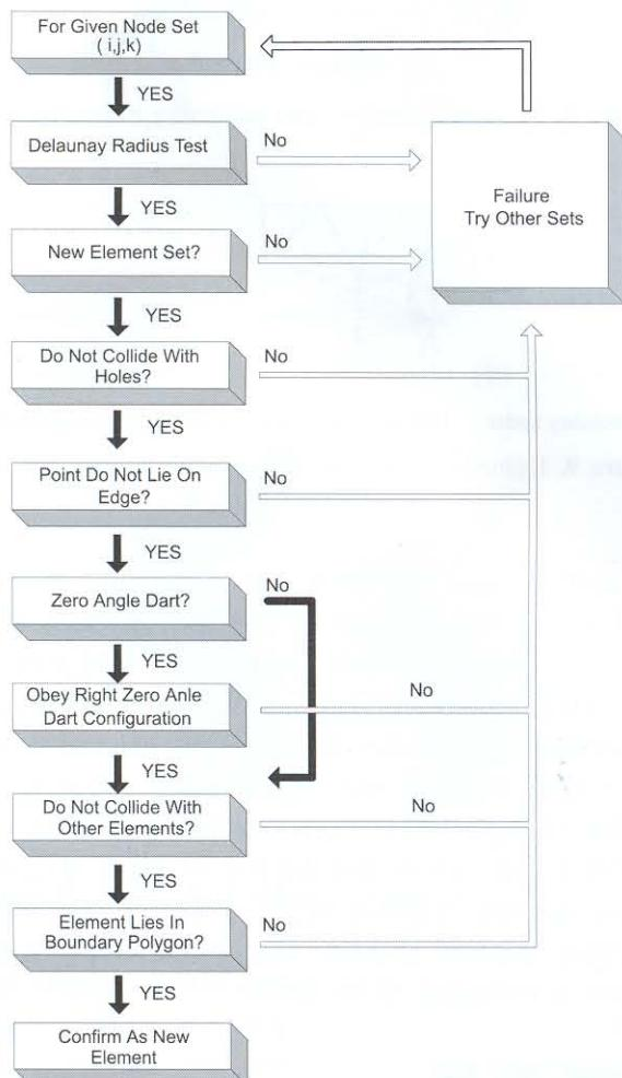
Figure 5. Triangulation procedure.
