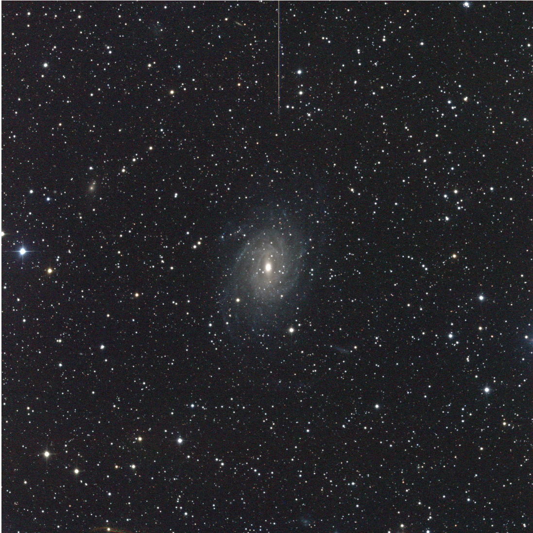
Figure 2.4. A color composite test image of NGC 6744 ( gri ) taken by STX16803 CCD. The field of view is 49'.4 \times 49'.4 . A feature on the top middle of the image is a bad pixel column.
