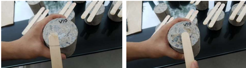
Figure 4.3 Lubricating process with wood stick
