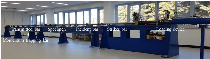
Figure 3.4 The SHPB system in Extreme Performance Testing Center
