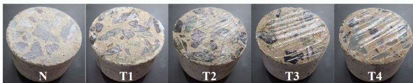
Figure 4.4 Lubricated specimens with Teflon for each amount of the lubricant
