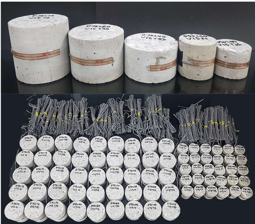
Figure 4.16 Prepared specimens for the concrete SHPB test
