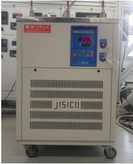
Figure 2.4. Thermostat water bath equipment and Schematic of formation of \frac{p_{H_2(g)}}{p_{H_2O(g)}} through thermostat water bath
