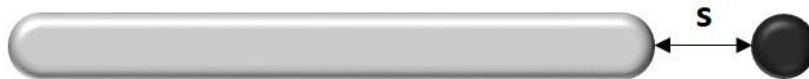
Figure 7.2 A system of a charged nanowire and a CNP. The separation distance s is varied in (a) the side direction and (b) the tip direction of the charged nanowire.
