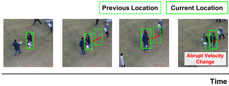
Figure 6. Tracking failure due to occlusion leads to large acceleration.
