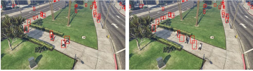
Figure 3. Example of object tracking error due to detection latency. Ideal detection result (left) and 1s delayed rendering result (right).
