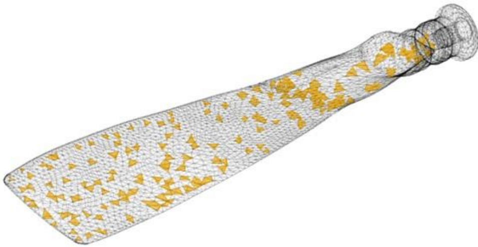
Fig. 5.14 Reduced number of meshes for the 54H60 propeller blade (166 selected elements).
