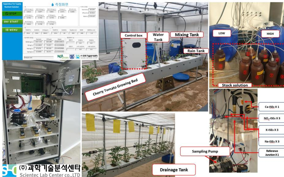
Figure 3.11 Schematic diagram of the evaluation test done while growing cherry tomato
