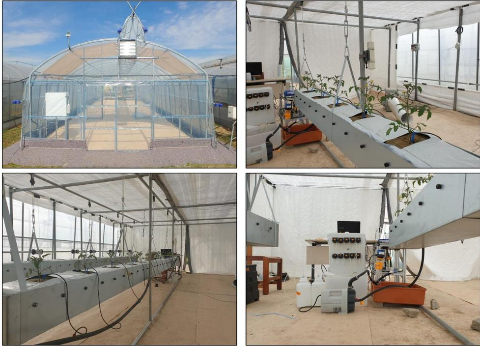
Figure 3.12 Na ion monitoring system applied to cherry tomato growing site
